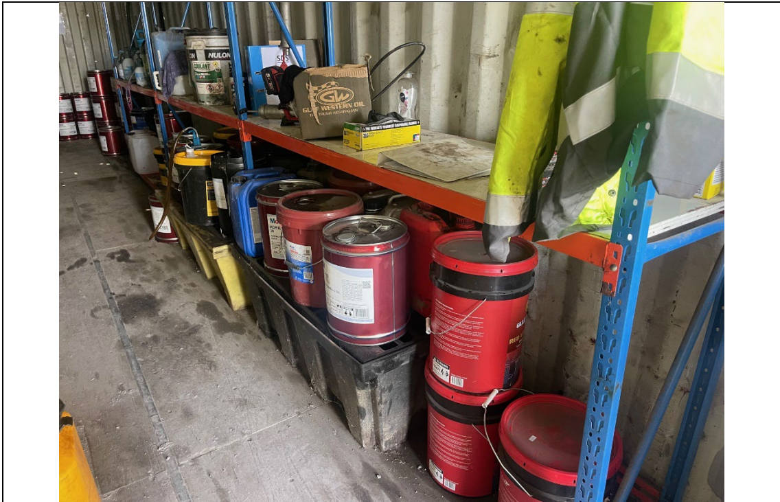
Photo 8 Chemical storage within a dedicated shipping container utilising bunds.
