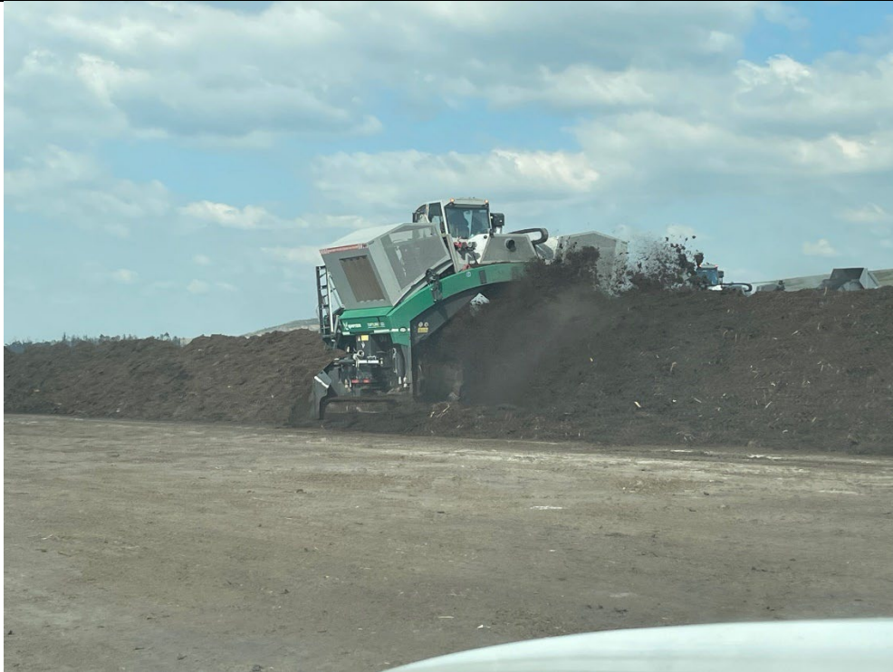
Photo 10 Bettergrow machinery mixing greenwaste with biosolid waste to form compost.
