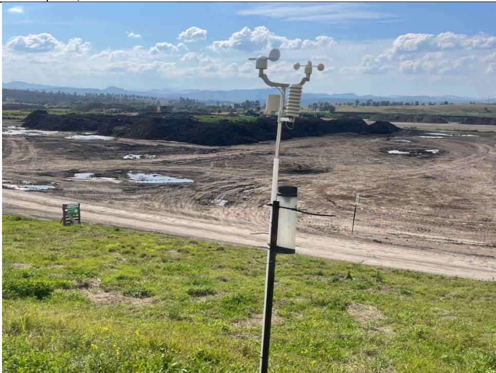
Photo 11 Onsite weather station with finished compost product in background.
