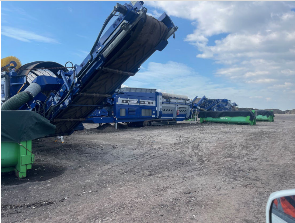
Photo 14 Screening process used to remove over-sized and plastic objects from the incoming green waste.
