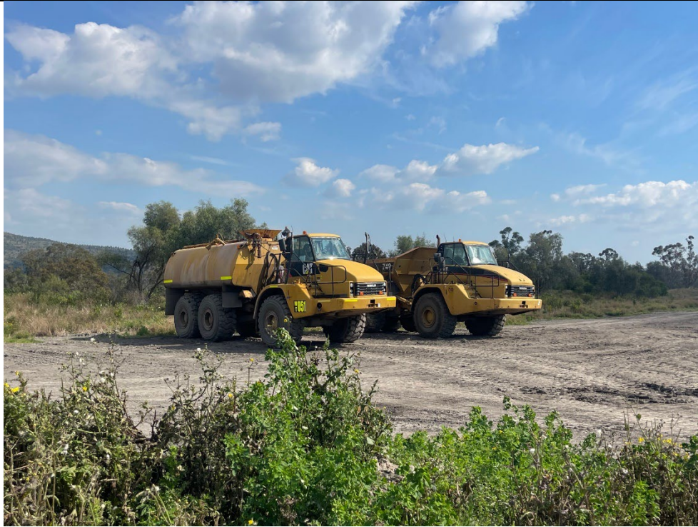
Photo 12 Dedicated water cart available on site. Water is pumped from the nearby AGL 'void 4'.
